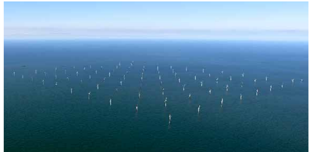
To obtain maximum capacity utilisation for each wind turbine, they have been erected 560 metres from one another. The 80 turbines have been installed to occupy a total area of 20 sq. km.
